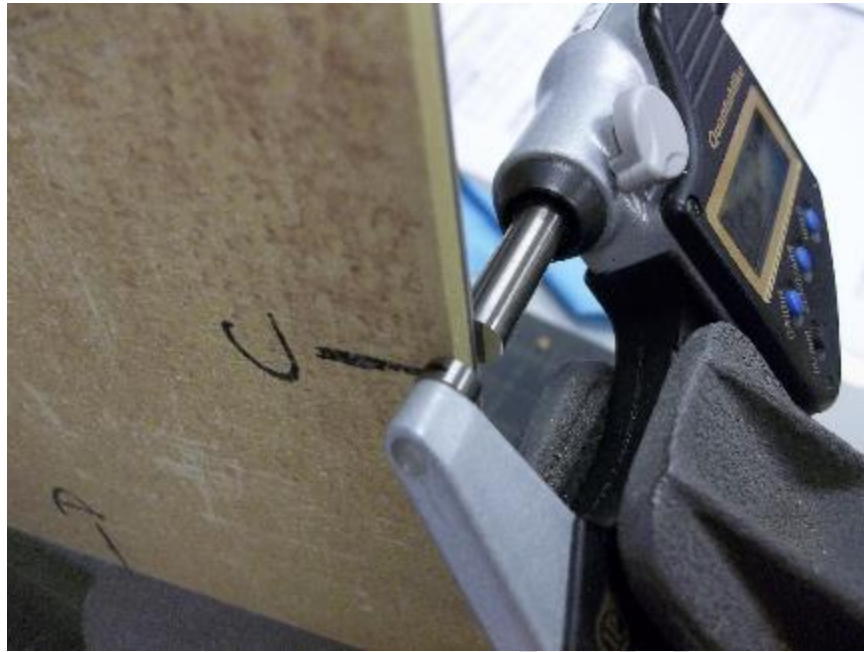
Photo No. 1 3.2 - Thickness Swell Measurement Detail (Typical)
