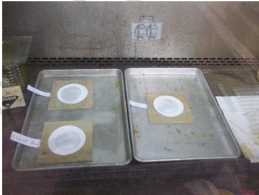
Photo No. 12 ASTM F1700 Sec. 6.8 - Resistance to Chemicals Test In-Progress
