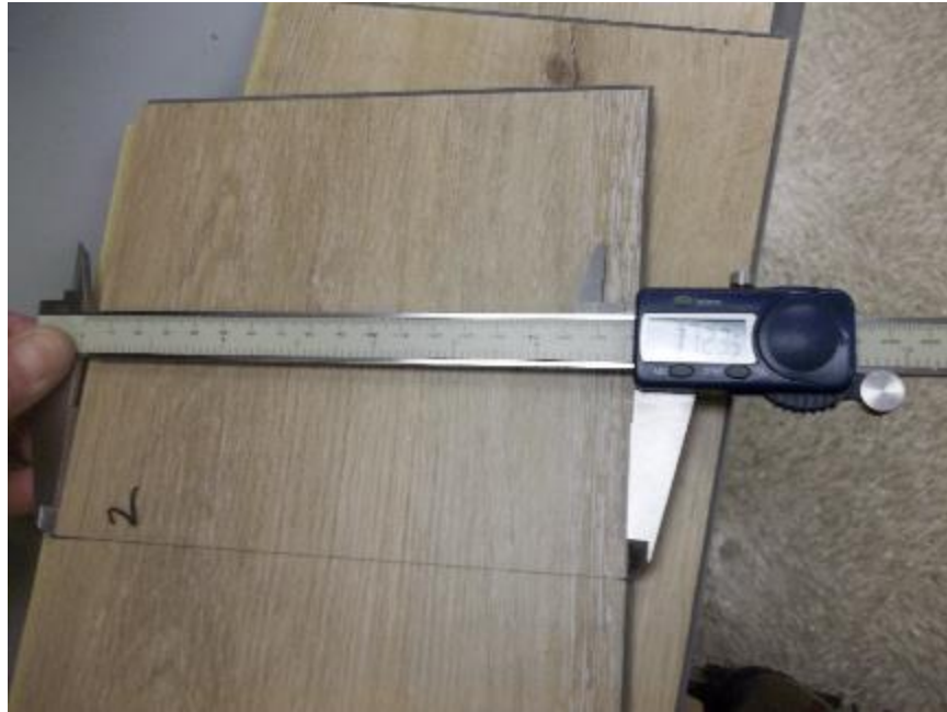
Photo No. 7 3.8 - Dimensional Tolerance Test In-Progress
