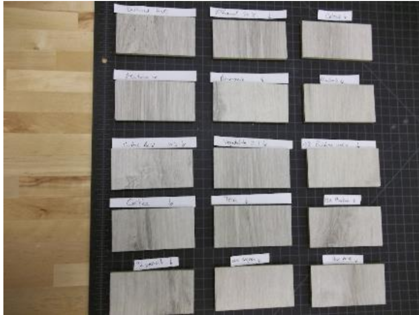
Photo No. 3 3.4 - Cleanability Stain Resistance Post-Test Results
