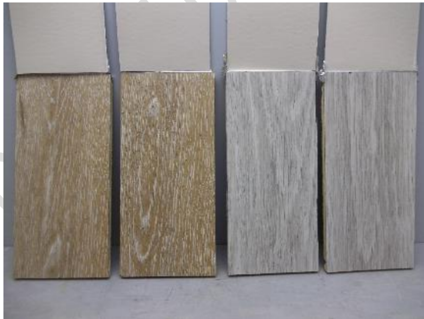
Photo No. 2 3.3 - Light Resistance Specimens Post-Test Results
