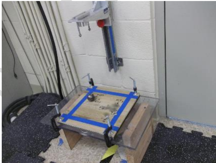
Photo No. 4 3.5 - Large Ball Impact Test Setup
