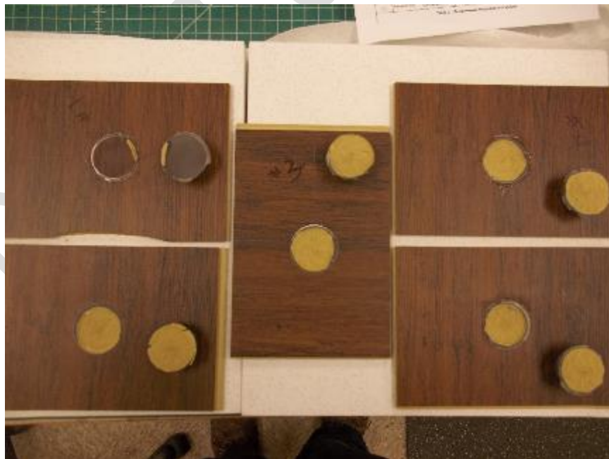
Photo No. 8 3.10 - Surface Bond Post-Test Specimen
