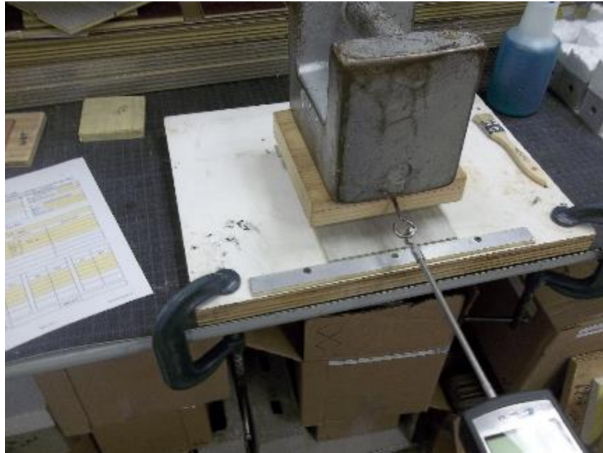
Photo No. 9 ASTM C1028 - Coefficient of Friction Testing Setup
