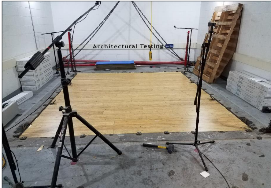
Source Room View of Test Specimen Installation
