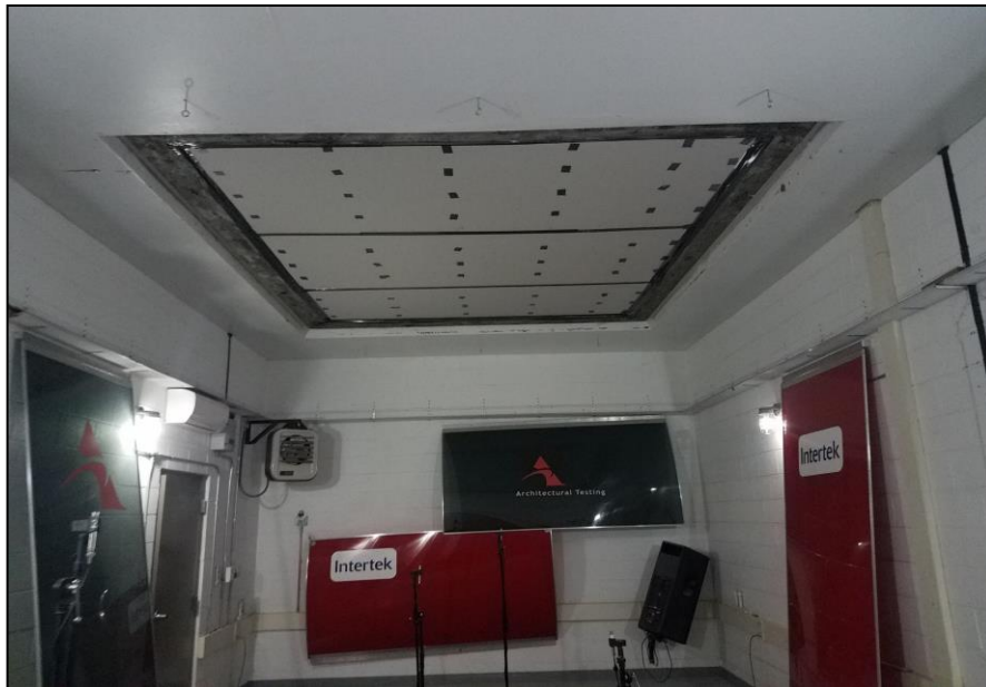
Receive Room View of Test Specimen Installation
