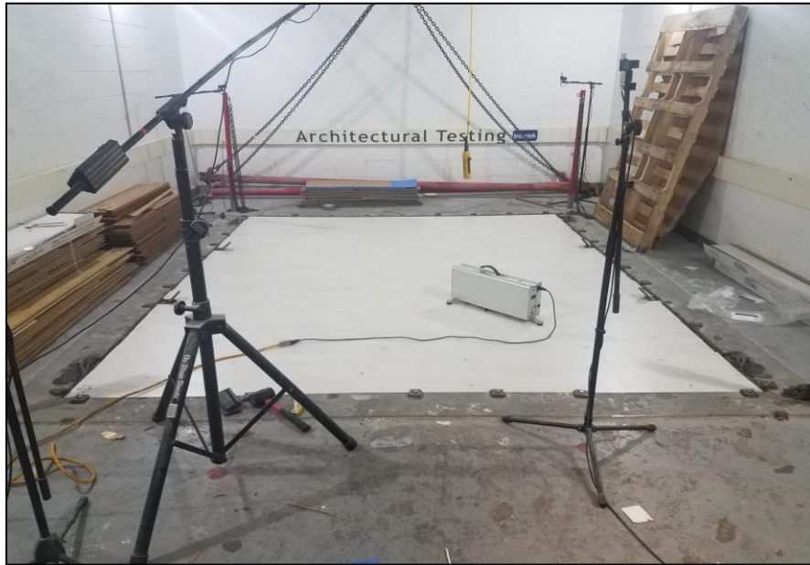
Source Room View of Test Specimen Installation
