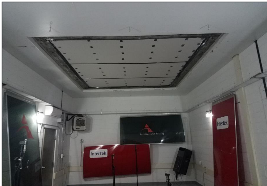
Receive Room View of Test Specimen Installation
