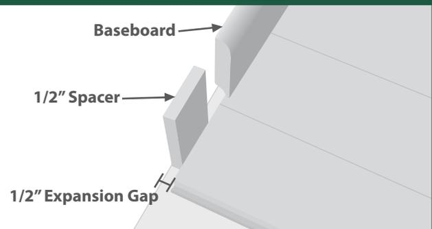
Leave at least 1/2" expansion spaces between flooring and ALL vertical objects (walls, cabinets, pipes, etc.) Large flooring runs may require additional expansion space. For floating floors, use transition moldings between rooms and doorways 3ft. or less. Undercut door jambs and casings to provide adequate expansion space. Do not screw or nail cabinetry or other permanent fixtures to a floating floor.
