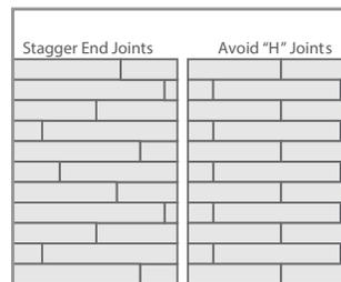
**Note: Although H joints do not void a warranty, they can decrease the overall structural strength of the flooring therefore Cali never recommends H joint installation.**
